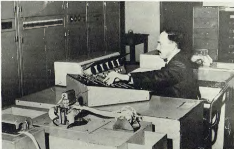
Pic 1. CSIRAC's control panel operation. The computer was fed coded punch tape. Pic 2. Operator on left uses a special ticker tape keyboard to punch out coded instruction tape for CSIRAC.
